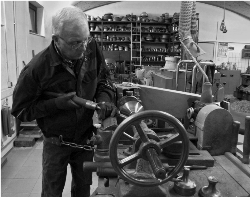
Christoph Müller in his workshop. At the beginning of the production process the chalices are a distinct red-orange colour because of the copper that is used
